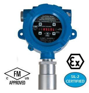
Factory Mutual (FM) Approval for performance, electrical safety and environmental parameters including Class I, Div. 1, Groups C, D and Class I, Zone 1, Group IIC. The 5100-28-IT is also SIL-2 Certified and meets NFPA-72 requirements for gas detectors.
