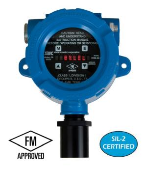
Factory Mutual (FM) Approval for performance, electrical safety and environmental parameters including Class I, Div. 1, Groups B, C, D and Class I, Zone 1, Group IIC, IP66. With a NEMA-4X enclosure standard, approved multiplexing, and approved six month calibration interval, cost of ownership is minimized at the acquisition, installation and operating stages
