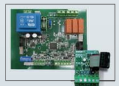
Expansion Kit RS482 Kit power board i-HB (for i-CHD units only)
