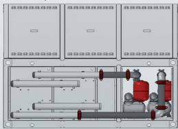
Configuration: 1 evaporator pump + 1 condenser pump
